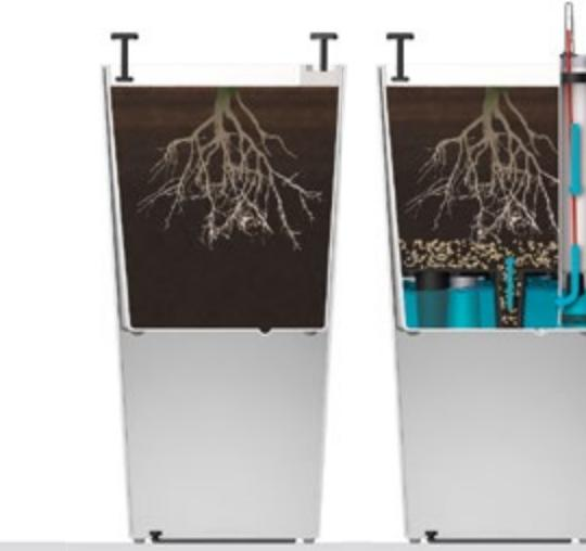
Hooks for comfortable removal of the inner pot
